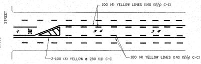
A MINIMUM OF TWO PAIRS OF TURN ARROWS SHALL BE USED, WHITE IN COLOR. ADDITIONAL PAIRS SHALL BE PLACED AT 60 m (200') TO 90 m (300') INTERVALS.
