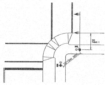
RECOMMENDED PUSHBUTTON LOCATIONS FOR ACCESSIBLE PEDESTRIAN SIGNALS SHALL BE IN ACCORDANCE WITH THE CURRENT MUTCO (SEE NOTE I). TO MEET MUTCO REQUIREMENTS, PEDESTRIAN SIGNAL PUSHBUTTONS MAY HAVE TO BE MOUNTED ON A SEPARATE POST.
