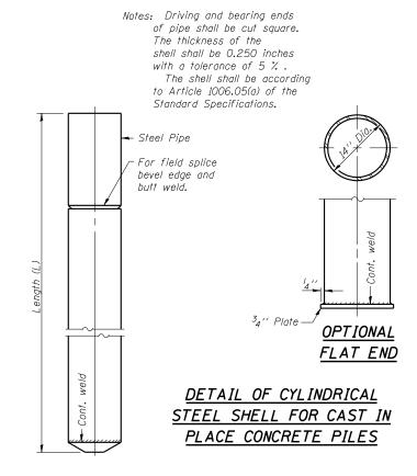
Note: Metal Shell Piles shall be according to ASTM A 252 Grade 3.
