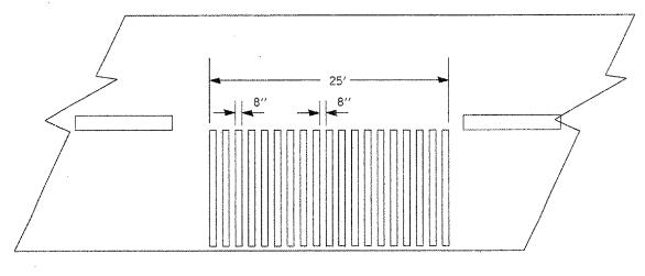
NOTE: THE 25-FOOT RUMBLE AREA HAS 8- INCH LENGTHS OF TREATED SURFACE STRETCHED ACROSS THE WIDTH OF APPROACH LANE, EACH SEPARATED BY 8 INCHES OF EXISTING PAVEMENT.
