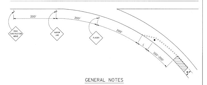
CONES AT 8 m (25')CENTERS FOR 105 m (350'). ADDITIONAL CONES MAY BE PLACED AT 15 m (50') CENTERS. WHEN DRUMS OR BARRICADES ARE USED. THE INTERVAL DEVICES MAY BE DOUBLED.
