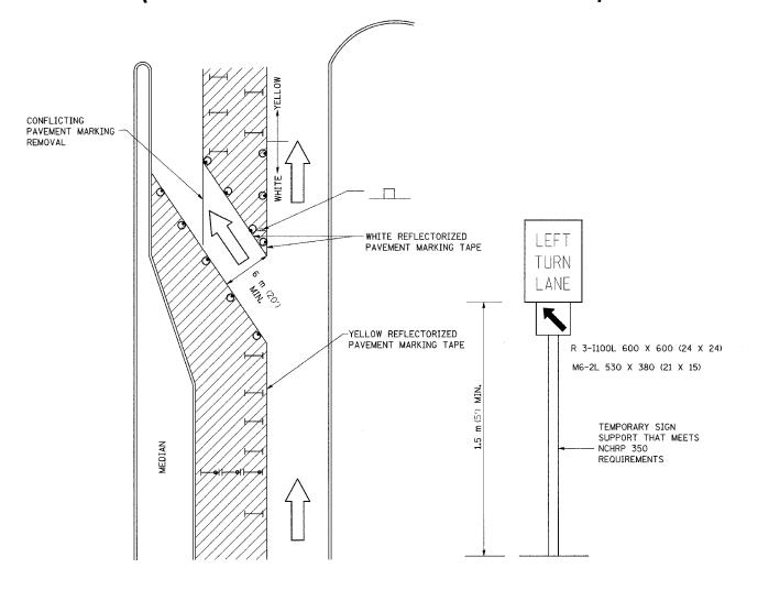
GENERAL NOTES CONES MAY BE SUBSTITUTED FOR BARRICADES OR DRUMS AT HALF THE SPACING
