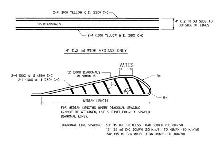
MEDIANS OVER 4' (1.2 m) WIDE -4 (100) YELLOW LINES (51/2 (140) C-C) -4 (100) YELLOW LINES (51/2 (140) C-C) ---2-4 (100) YELLOW @ 11 (280) C-C A MINIMUM OF TWO PAIRS OF TURN ARROWS SHALL BE USED, WHITE IN COLOR.
