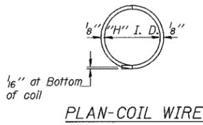
ILLINOIS COIL-LOCK ANCHOR BOLT
