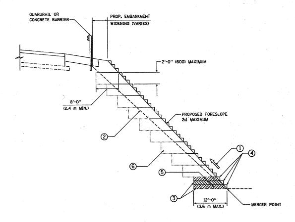
TYPICAL BENCHING DETAIL FOR EMBANKMENT
