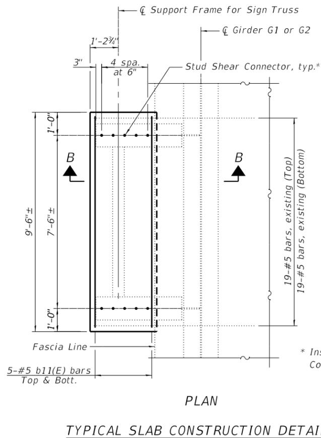
\* Install 5 Each 3/4" Ø x 4" Stud Shear Connector along C/C of Beam.
