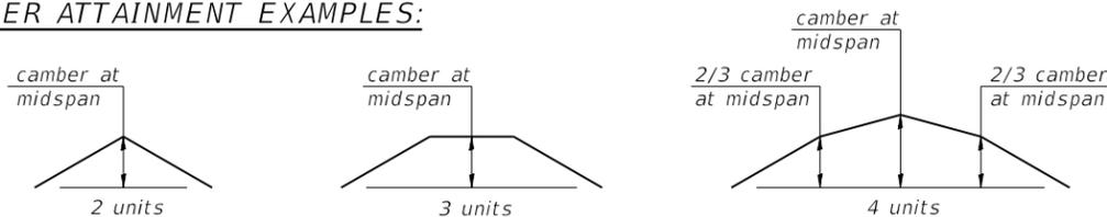
Camber shown is for fabrication only, measured with truss fully supported. (No-load condition)
