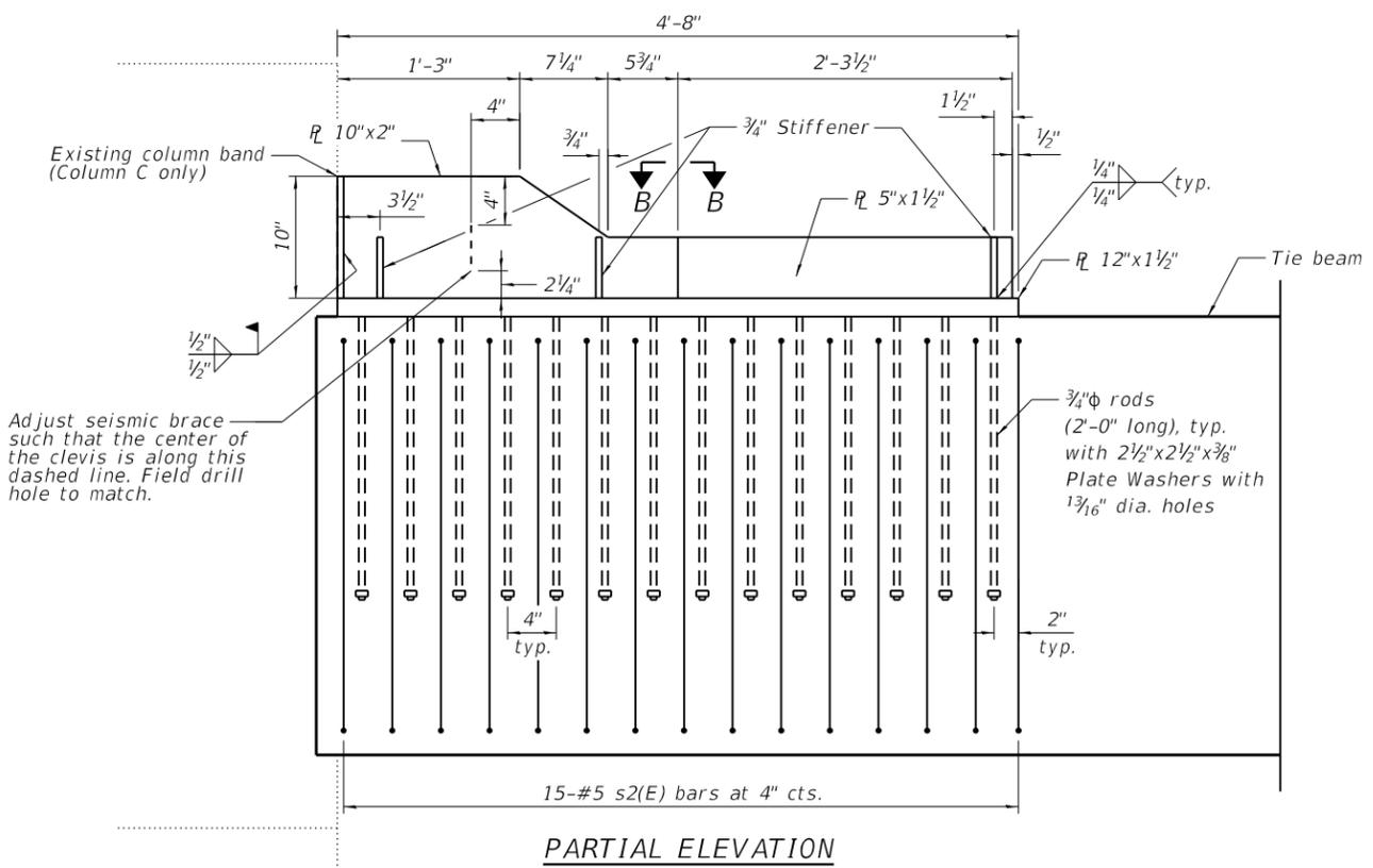
Adjust seismic brace such that the center of the clevis is along this dashed line. Field drill hole to match.
