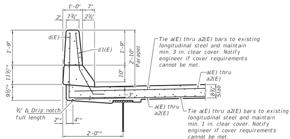
SECTION THRU PARAPET
