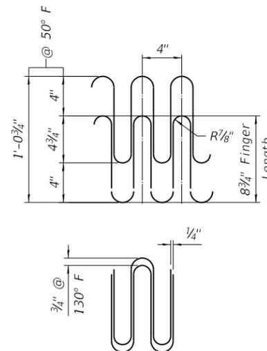
**JOINT OPENING AND GEOMETRY DETAIL**
