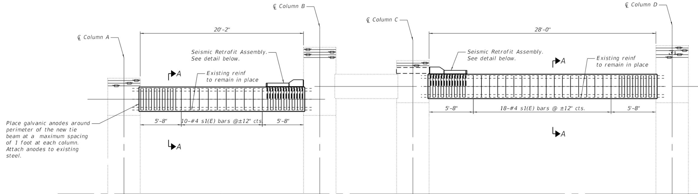
Place galvanic anodes around perimeter of the new tie beam at a maximum spacing of 1 foot at each column. Attach anodes to existing steel.
