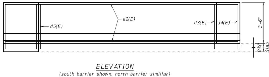
\*Drill and epoxy #5 d3(E), d4(E), and d5(E) bars according to epoxy manufacturer's recommendations. Maximum depth of hole shall not exceed 6". Anchoring epoxy shall be approved by engineer.
