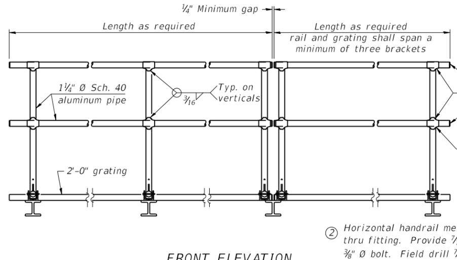
1 Install standard force-fit end caps or weld 1/8" end plates with 1/8" c.f.w. and grind smooth. (All rail ends)
