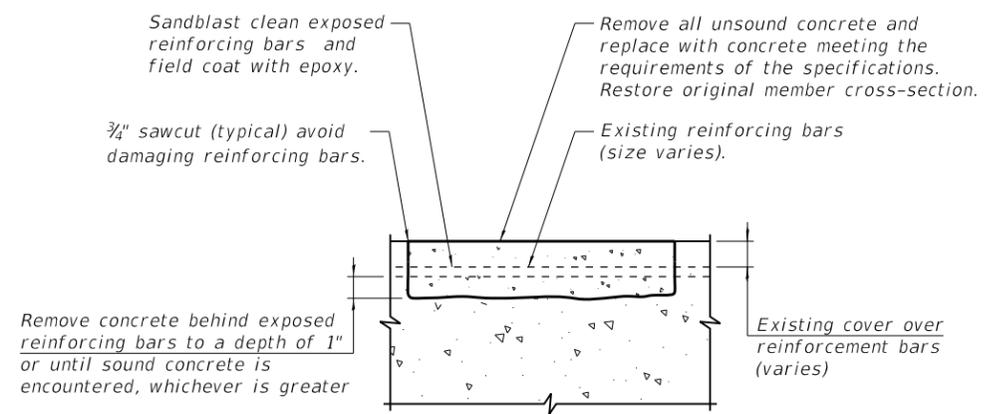
**HORIZONTAL SURFACE REPAIR (PARTIAL DEPTH)**
