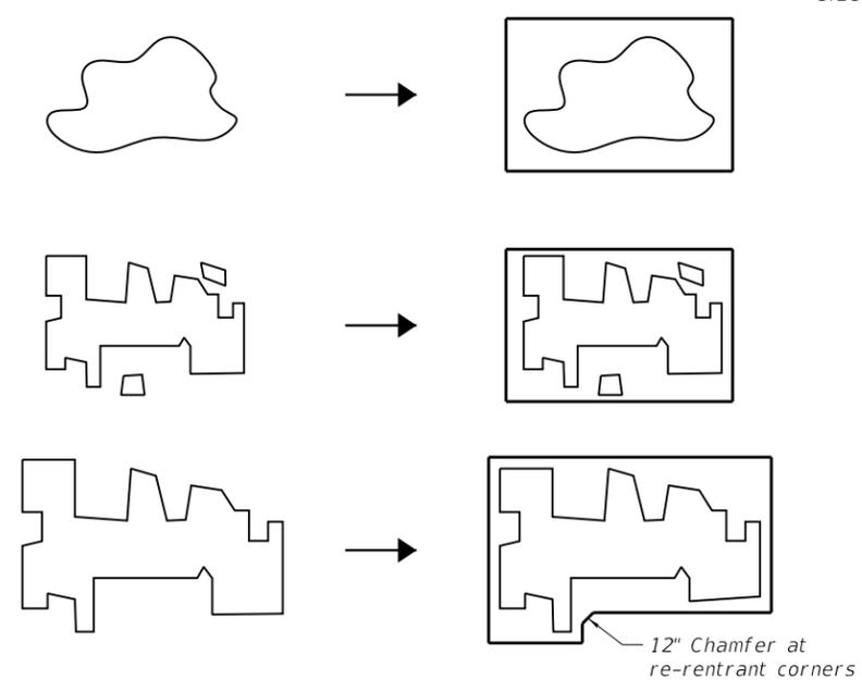
**TYPICAL CONCRETE REPAIR GEOMETRY**
