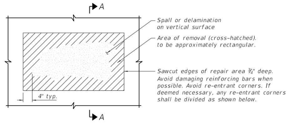
**VERTICAL SURFACE REPAIR DETAIL**
