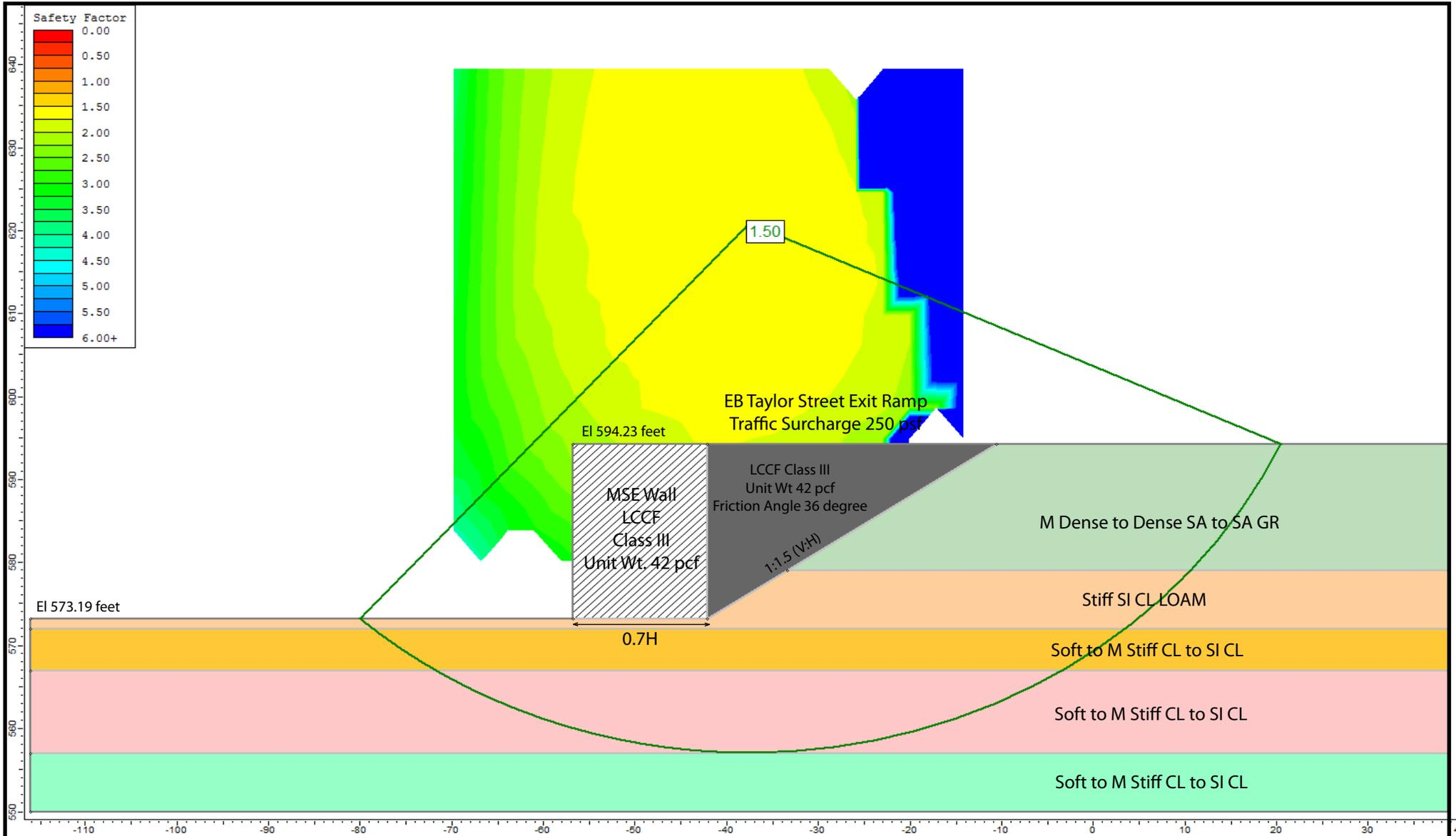
Undrained Analysis for MSE Wall at Station 7326+25.98, Ref Borings 10-RWB-09, 16-RWB-04A, 16-RWB-04B, 16-RWB-05 and VST-07
