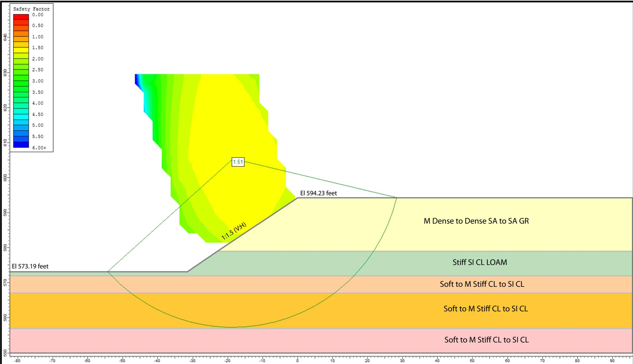
Undrained Analysis for Excavation at Station 7326+25.98, Ref Borings 10-RWB-09, 16-RWB-04A, 16-RWB-04B, 16-RWB-05 and VST-07
