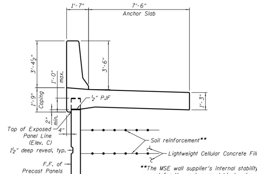
**SECTION THRU PARAPET AND ANCHORAGE SLAB**
