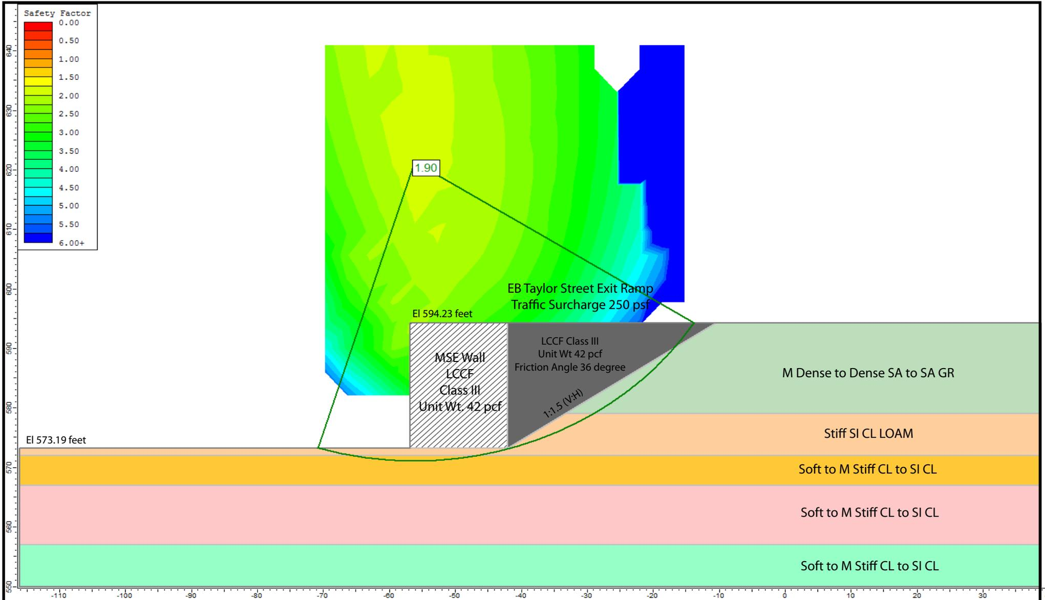
Drained Analysis for MSE Wall at Station 7326+25.98, Ref Borings 10-RWB-09, 16-RWB-04A, 16-RWB-04B, 16-RWB-05 and VST-07
