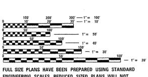
ENGINEERING SCALES, REDUCED SIZED PLANS WILL NOT CONFORM TO STANDARD SCALES. IN MAKING MEASUREMENTS ON REDUCED PLANS, THE ABOVE SCALES MAY BE USED.
