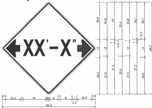
W12-2 - Hortzontal Clearance Sign 48.0" across sides, 1.9" Radius, 0.8" Border, 0.5" Indent, Black on Orange: Standard Arrow Custom 10.4" X 8.1" 180° Black 11 Inch D Series Lettering: Standard Arrow Custom 10.4" X 8.1" 0°
