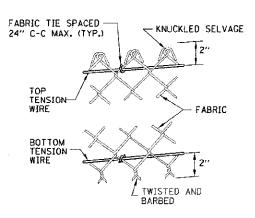
METHOD OF TYING FABRIC TO TENSION WIRES
