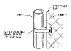
STRETCHER BARS SHALL BE GALVANIZED FLAT STEEL BAR NOT LESS THAN 1/4"×3/4" AND THE STRETCHER BAR BANDS SHALL BE GALVANIZED FLAT STEEL BAR NOT LESS THAN 1/8"× 1" WITH A 3/8" GALVANIZED CARRIAGE BOLT.
