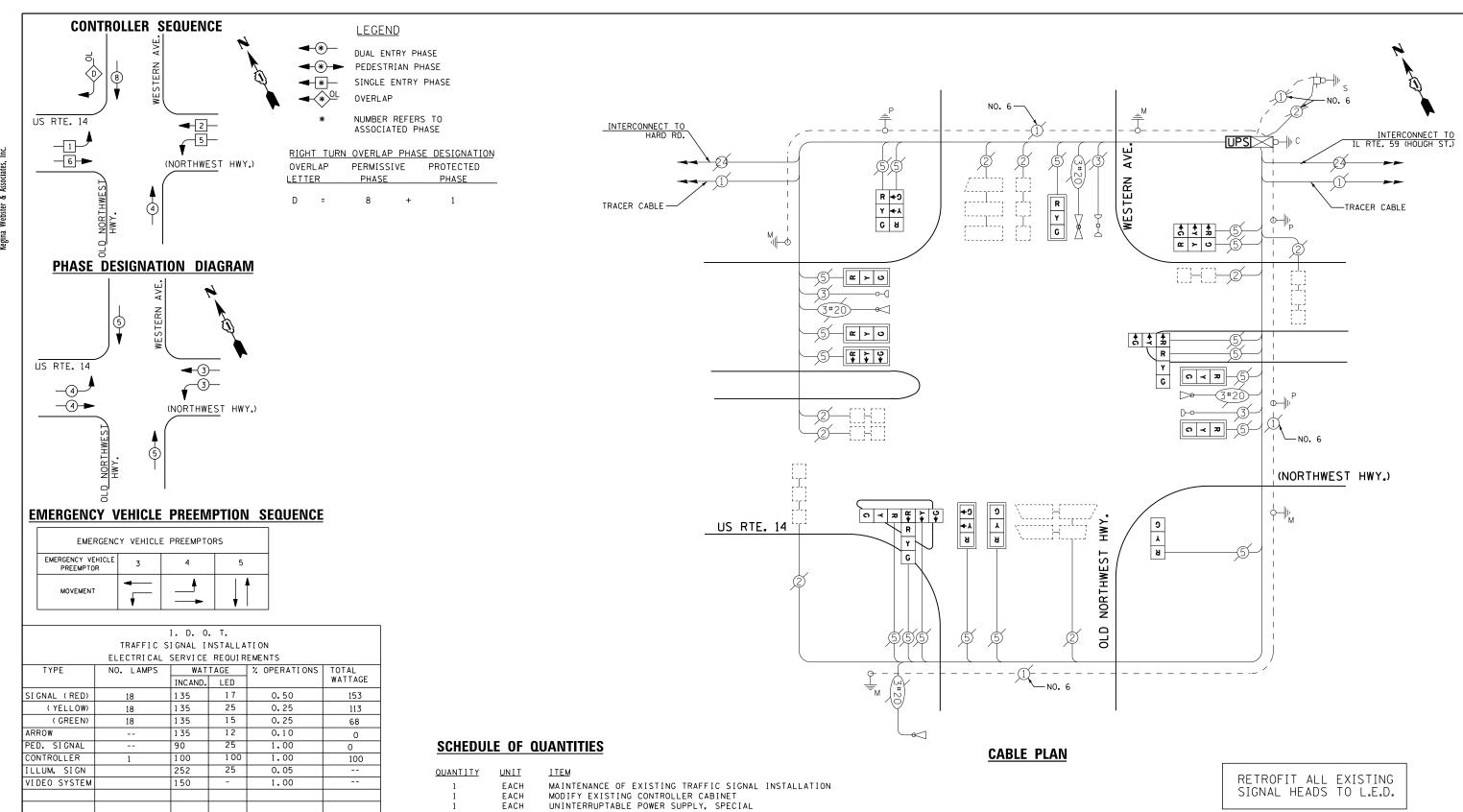
EACH SIGNAL HEAD, LED, 1-FACE, 3-SECTION, BRACKET MOUNTED, RETROFIT SIGNAL HEAD, LED, 1-FACE, 3-SECTION, MAST ARM MOUNTED, RETROFIT EACH SIGNAL HEAD, LED, 2-FACE, 3-SECTION, BRACKET MOUNTED, RETROFIT EACH SIGNAL HEAD, LED, 3-FACE, 3-SECTION, BRACKET MOUNTED RETROFIT
