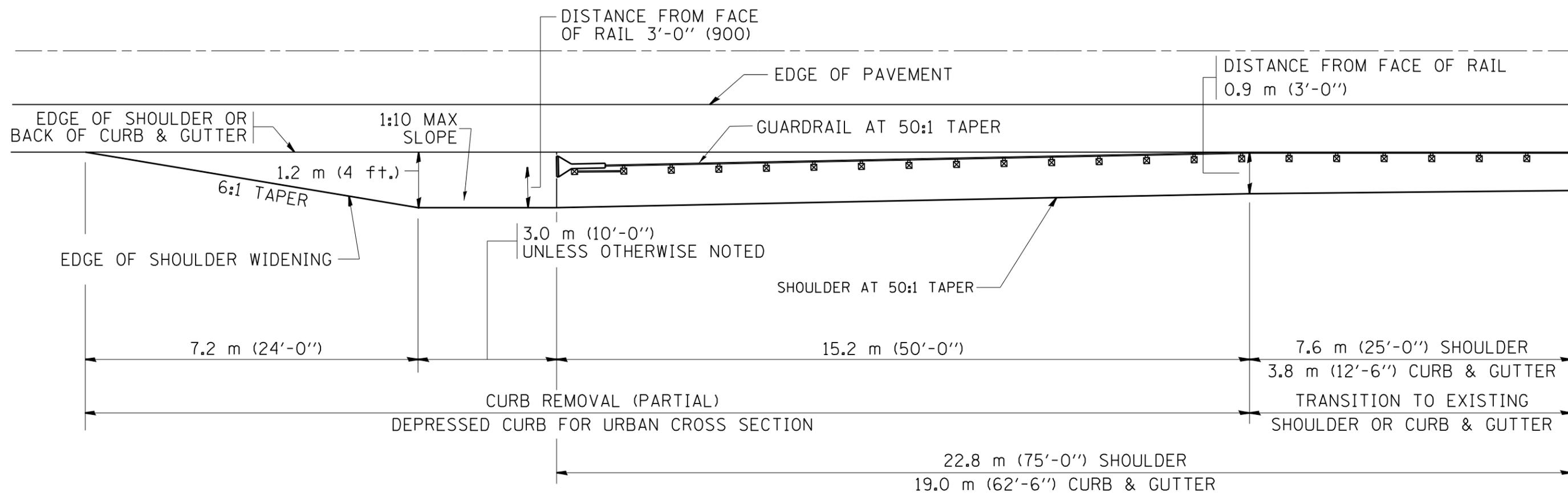
NOTES: THE CONTRACTOR SHALL VERIFY THE TYPE/HEIGHT OF GUARDRAIL IN-PLACE BEFORE ORDERING THE NEW TERMINAL SECTION. COST INCLUDED WITH THE COST OF THE TERMINAL. THE TERMINAL SECTION HEIGHT TO BE PLACED MUST MATCH THE HEIGHT OF THE IN-PLACE GUARDRAIL.
