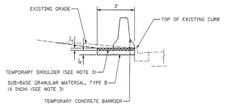
TEMPORARY CONCRETE BARRIER PLACEMENT
