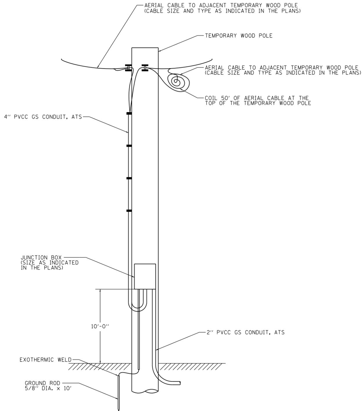
JUNCTION BOX ATTACHED TO WOOD POLE INSTALLATION DETAIL
