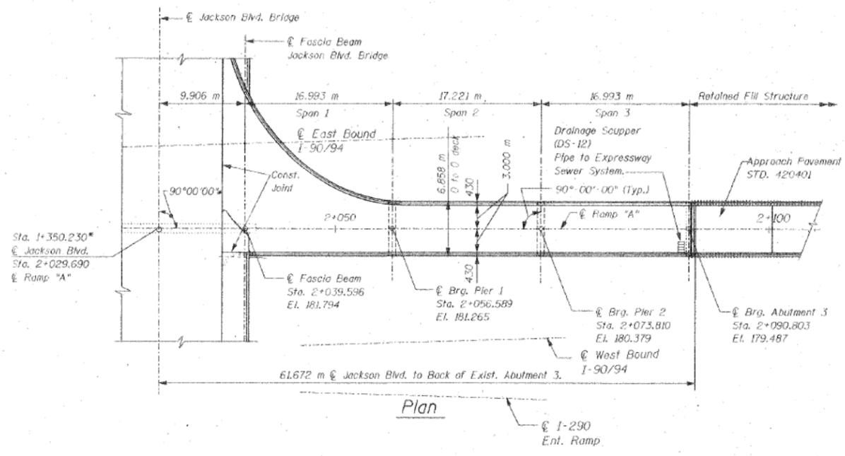
\* Stationing and angle for ramp location is based on the plans of the existing structure. The contractor must verify the location prior to fabrication of any material.
