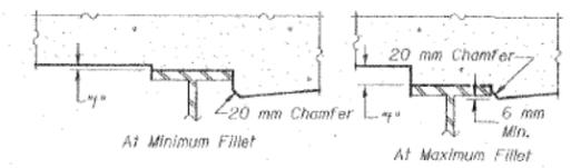
To determine "f": After all structural steel has been erected, elevations of the top flanges of the beams shall be taken at intervals shown above. These elevations subtracted from the "Theoretical Grade Elevations Adjusted for Dead Load Deflection" shown on S6 through S9, minus slab thickness, equals the fillet heights "f" above top flange of beams.
