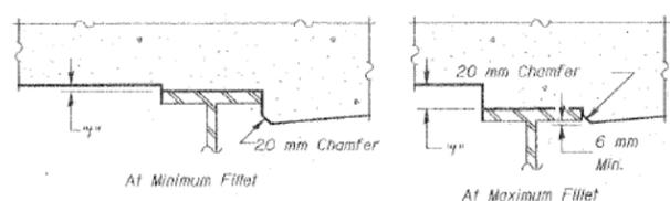
To determine "f": After all structural steel has been erected, elevations of the top flanges of the beams shall be taken at locations shown above. These elevations subtracted from the "Theoretical Grade Elevations Adjusted For Dead Load Deflection" shown below, minus slab thickness, equals the fillet heights "f" above top flange of beams.
