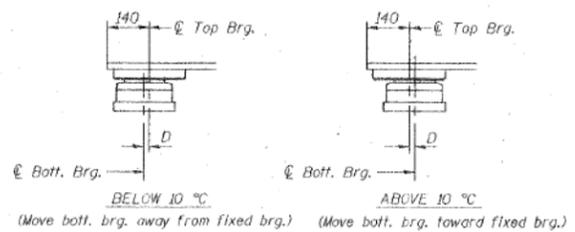
D = 1 mm per each 10 m of expansion for every 8 °C temp. change from the normal temp. of 10 °C.
