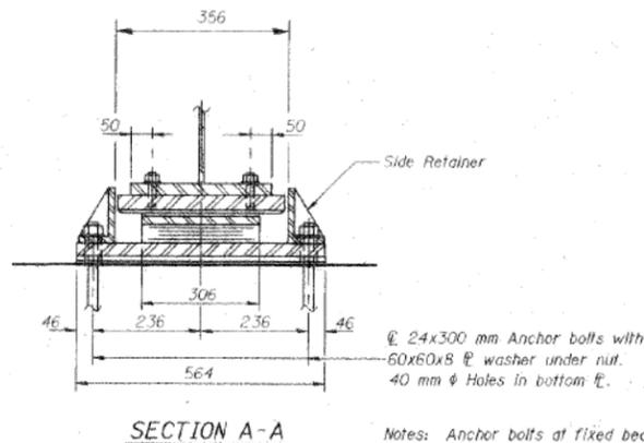
Notes: Anchor bolts at fixed bearings may be built into the masonry. See Sheet S-37 for Anchor Bolt Installation. All dimensions are in millimeters (mm) except as noted.
