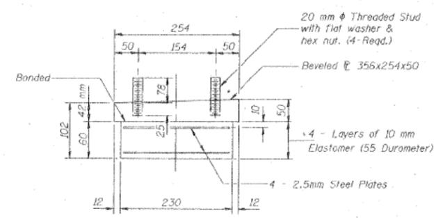
**BEARING ASSEMBLY EAST ABUTMENT**
