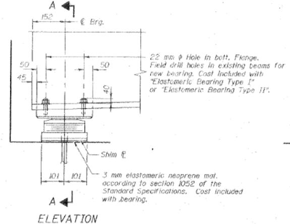
**TYPE II ELASTOMERIC EXP. BRG. WEST ABUTMENT**
