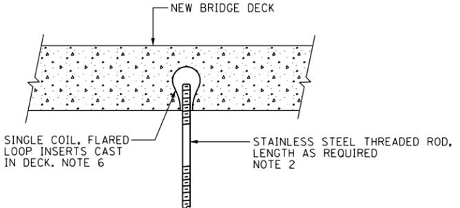
**NEW BRIDGE DECK THREADED ROD INSTALLATION ANCHOR DETAILS**
