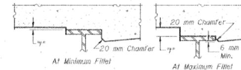
To determine "f": After all structural steel has been erected, elevations of the top flanges of the beams shall be taken at intervals shown above. These elevations subtracted from the "Theoretical Grade Elevations Adjusted for Dead Load Deflection" shown below, minus slab thickness, equals the fillet heights "f" above top flange of beams.
