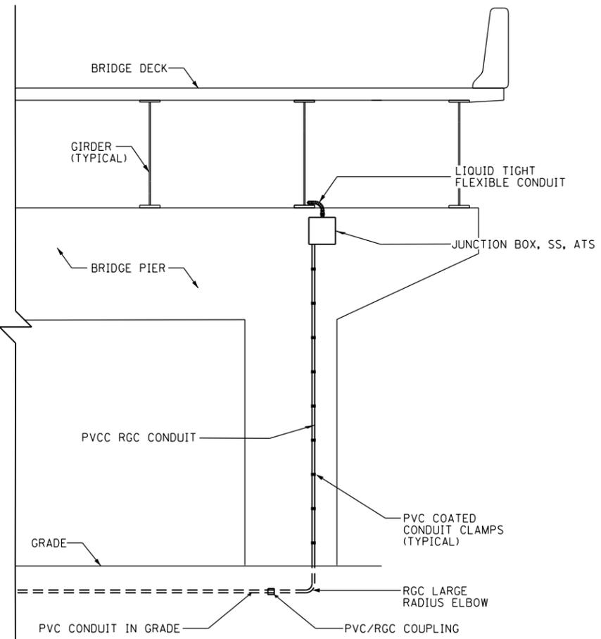
**VERTICAL CONDUIT ATTACHED TO STRUCTURE DETAIL**
