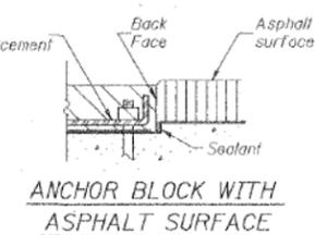
ANCHOR BLOCK WITH ASPHALT SURFACE
