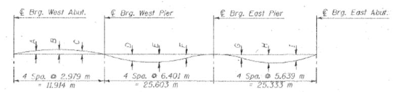
**Note:** The above deflections are not to be used in the field if the engineer is working from the grade elevations adjusted for dead load deflections as shown below. All dimensions are in millimeters (mm) except as noted. All offsets are in meters.
