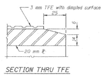
Note: The 3 mm TFE sheet shall be bonded directly to the top steel plate with a two-component, medium viscosity epoxy resin, conforming to the requirements of the Federal Specification MMM-A-134, Type I. The bond agent shall be applied on the full area of the contact surfaces.
