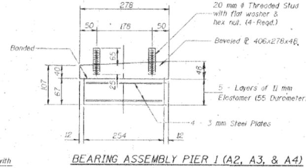
BEARING ASSEMBLY PIER 1 (A2, A3, & A4)
