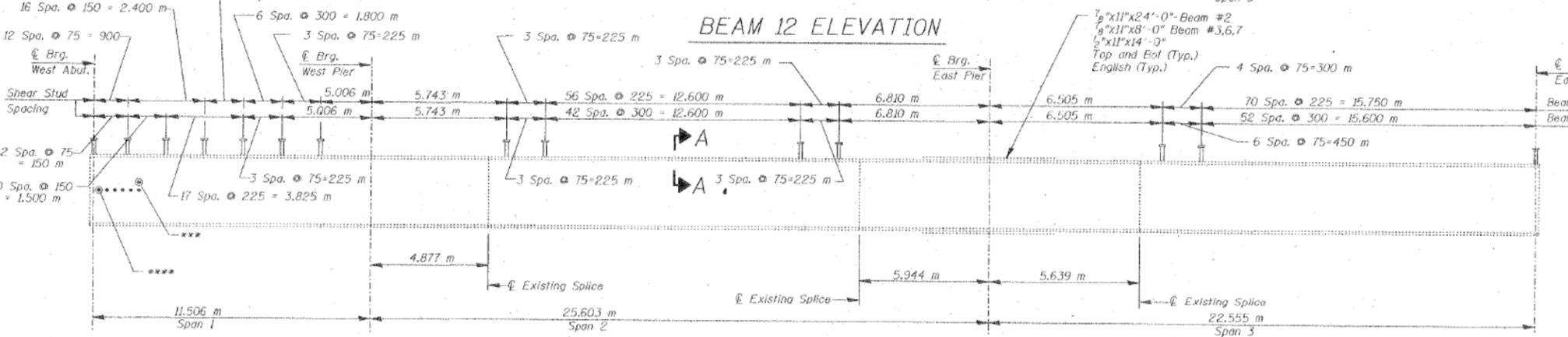
ELEVATION OF EXISTING BEAMS
