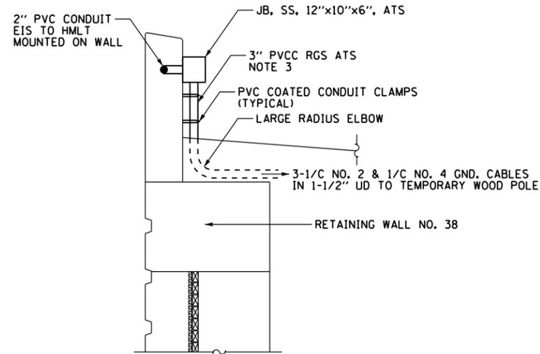
RETAINING WALL NO. 38 CONDUIT ROUTING DETAIL
