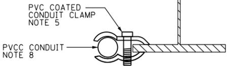
**CONDUIT BEAM CLAMPED INSTALLATION DETAIL**
