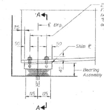
**TYPE I ELASTOMERIC EXP. BRG. EAST ABUTMENT**
