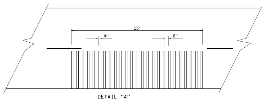
**NOTE:** THE 25 FEET RUMBLE AREA HAS 4" WIDE GROOVES SAWED INTO THE PAVEMENT, SEPARATED BY 8" OF EXISTING PAVEMENT. THE SAW CUTS SHALL EXTEND 12" INTO THE SHOULDER TO ALLOW FOR DRAINAGE.
