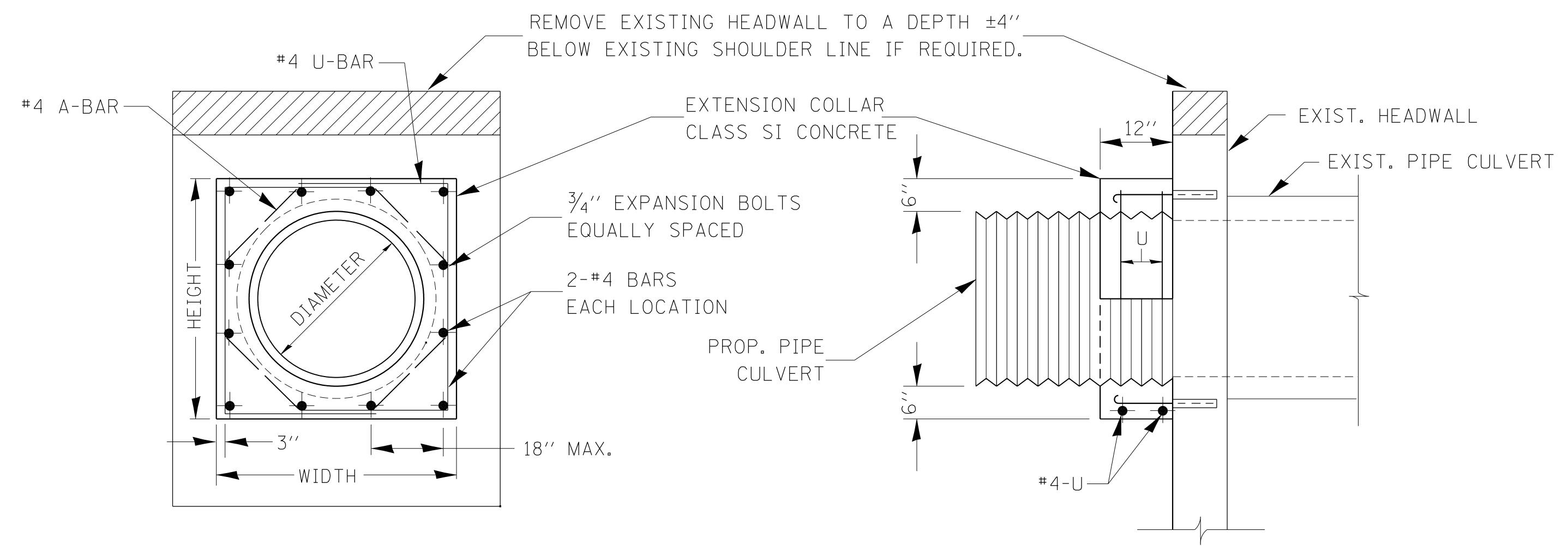
EXPANSION BOLTS SHALL CONSIST OF SELF DRILLING EXPANSION SHIELDS AND  $\frac{3}{4}$ " DIA. HOOKED BOLTS. HOOKED BOLTS SHALL EXTEND A MINIMUM OF 9" INTO NEW CONCRETE.
