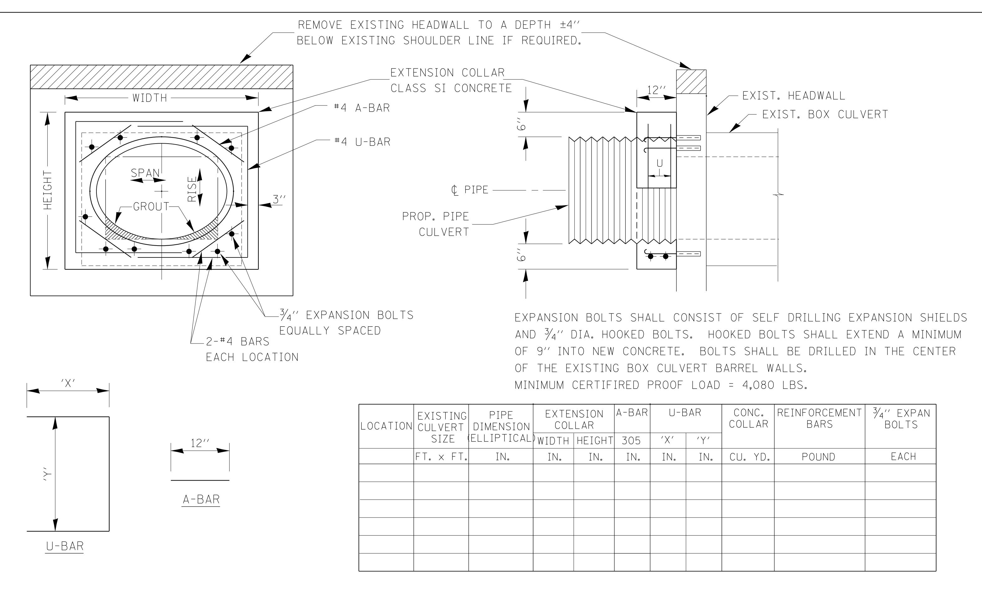
COLLAR DETAIL (ELLIP. CMP EXTENSION OF BOX CULVERT)
