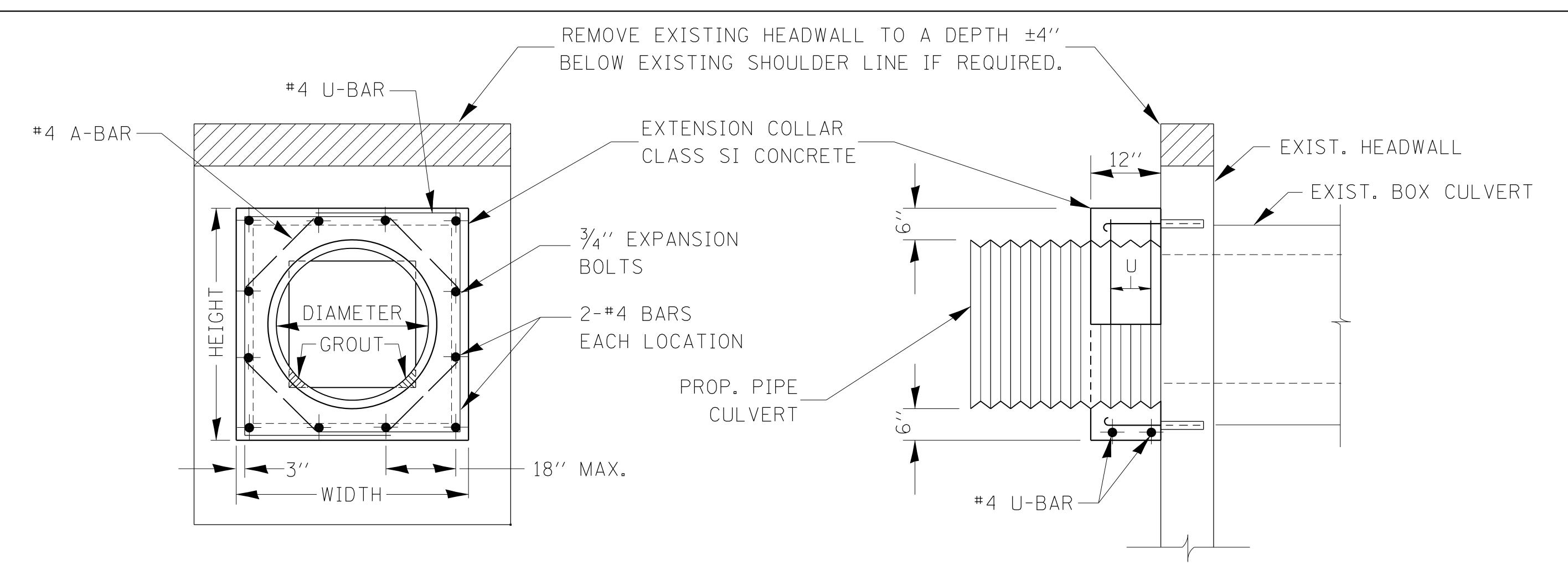
EXPANSION BOLTS SHALL CONSIST OF SELF DRILLING EXPANSION SHIELDS AND  $\frac{3}{4}$ " DIA. HOOKED BOLTS. HOOKED BOLTS SHALL EXTEND A MINIMUM OF 9" INTO NEW CONCRETE. BOLTS SHALL BE DRILLED IN THE CENTER OF THE EXISTING BOX CULVERT BARREL WALLS. MINIMUM CERTIFIRED PROOF LOAD = 4,080 LBS.
