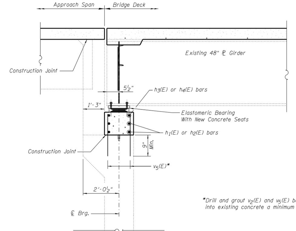
\*Drill and grout v<sub>2</sub>(E) and v<sub>5</sub>(E) bars into existing concrete a minimum of 9".
