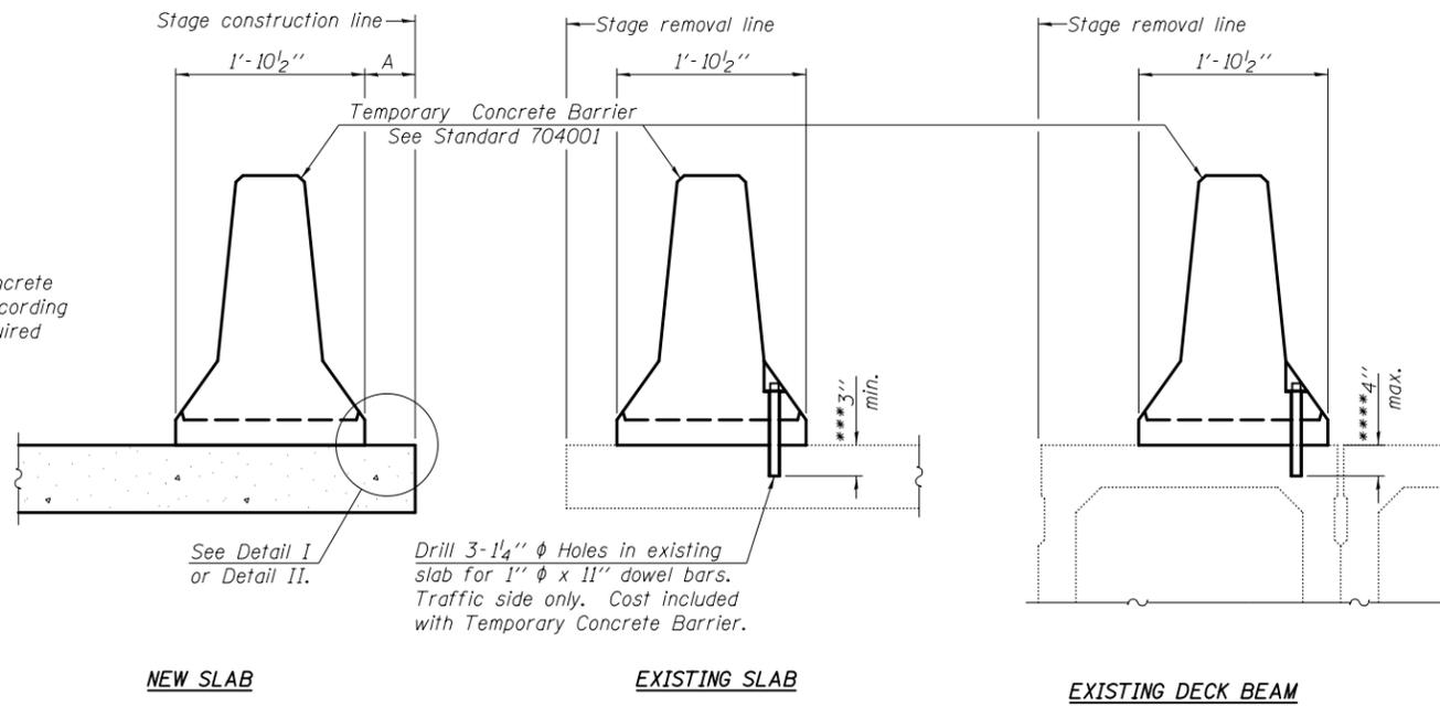
Drill 3-1 1/4"  $\phi$  Holes in existing slab for 1"  $\phi$  x 11" dowel bars. Traffic side only. Cost included with Temporary Concrete Barrier.
