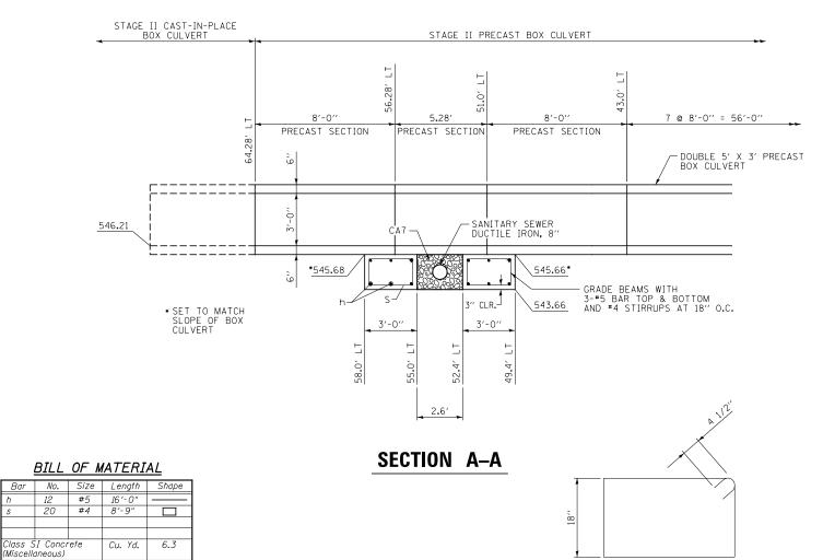
PLAN AT BOX CULVERT CROSSING OF SANITARY SEWER STA 6039+06.52
