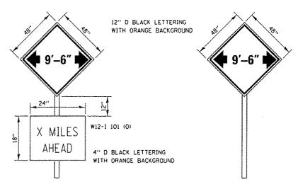
TO BE POST MOUNTED. TWO SIGNS REQUIRED.ONE IN THE WBL JUST SOUTH OF THE US 52 INTERSECTION, THE OTHER SIGN 1/2 MILE NORTH OF I-80 IN THE EBL
