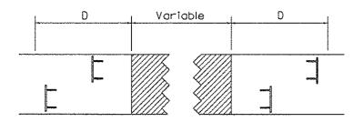
Type III Barricades and R11-4-4830 signs shall be as shown in "Road Closed To Thru Traffic" detail on Highway Standard 701901. If the distance "D" exceeds 2000' an additional set of barricades and R11-4-4830 shall be placed at each end of the work area.
