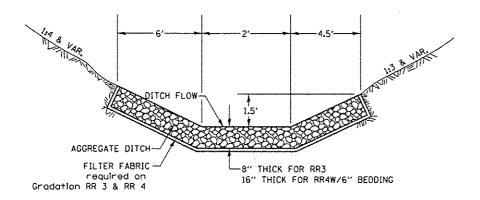
THIS WORK SHALL BE DONE IN ACCORDANCE WITH SECTION 281. AGGREGATE DITCH WILL BE MEASURED FOR PAYMENT IN PLACE AND THE AREA COMPUTED IN SQUARE YARDS OF ACTUAL SURFACE AREA.
