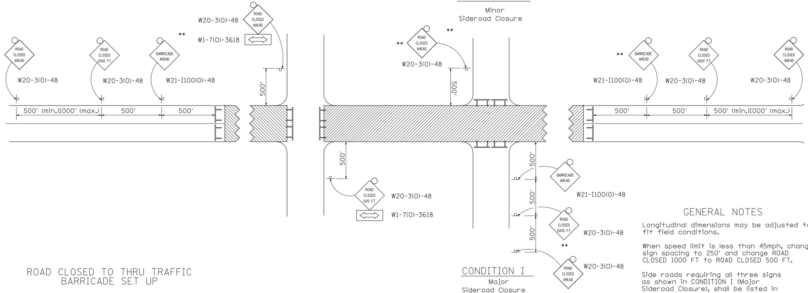
ROAD CLOSED TO THRU TRAFFIC BARRICADE SET UP
