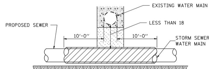
PROVIDE ADEQUATE SUPPORT FOR EXISTING WATER MAIN TO PREVENT DAMAGE DUE TO SETTLEMENT OF SEWER TRENCH
