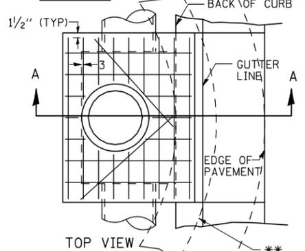
\*\* WHEN INLET IS CONSTRUCTED IN RETURN, THE TOP OF SLAB SHALL CONFORM TO THE RADIUS OF THE RETURN.
