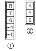
SIGNAL HEAD LOCATION AS DIRECTED BY ENGINEER AND TO BE ADJUSTED DURING STAGING ALSO AS DIRECTED BY THE ENGINEER.
