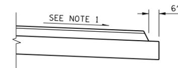
**TEMPORARY PAVEMENT DETAIL - STAGE 1**
