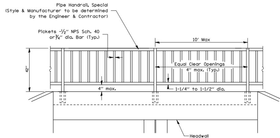
**PIPE HANDRAIL, SPECIAL – FOR HEADWALL**
