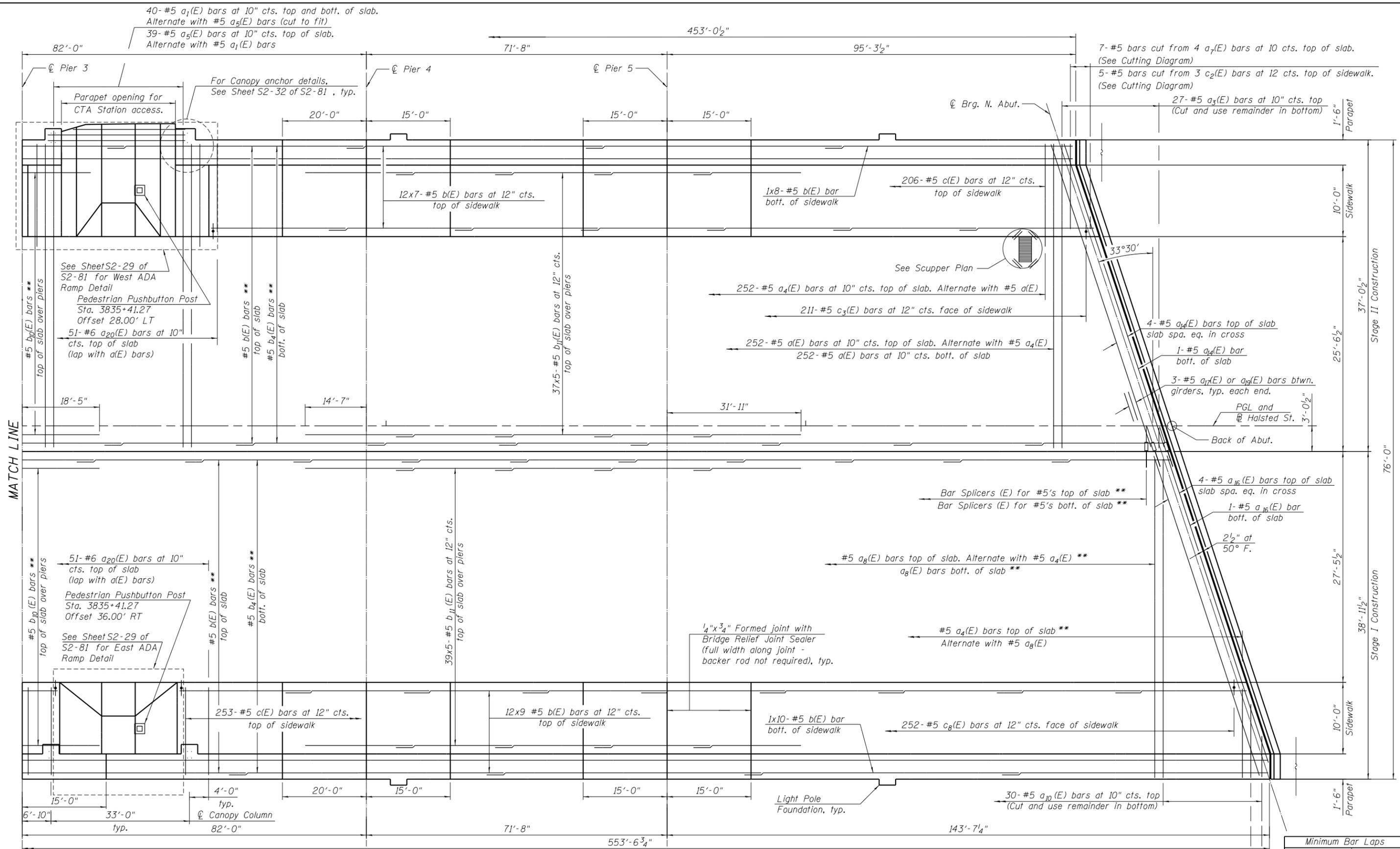
**Note:** Dimensions are based on a Rolled Rail Strip Seal joint. If the contractor elects to use the Welded Rail Strip Seal joint, deck dimensions may require adjustments to satisfy details on Sheet S2-41 of S2-81.
