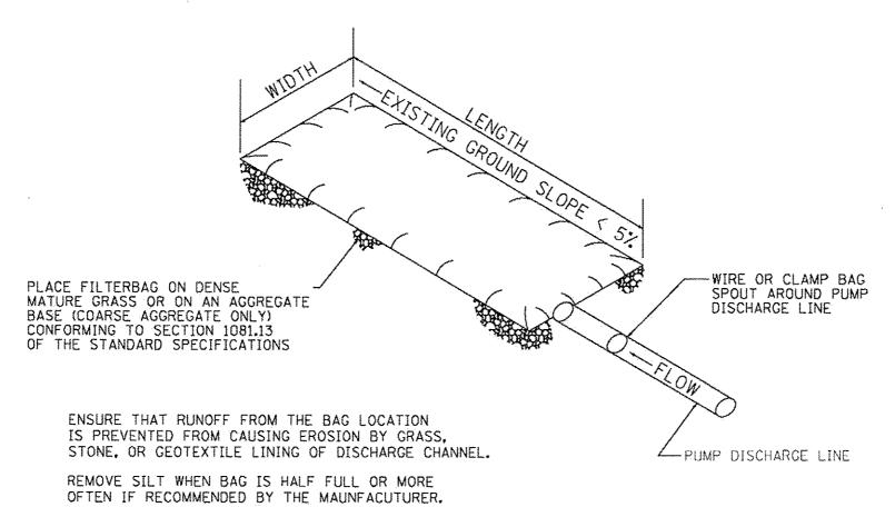
DISPOSE OF SILT BY TRANSPORTING THE FILLED BAG TO DISPOSAL AREA. SLIT THE BAG, BLEND SILT INTO EXISTING TOPOGRAPHY, SEED AND MULCH
