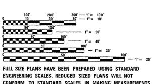
CONFORM TO STANDARD SCALES. IN MAKING MEASUREMENTS ON REDUCED PLANS, THE ABOVE SCALES MAY BE USED.
