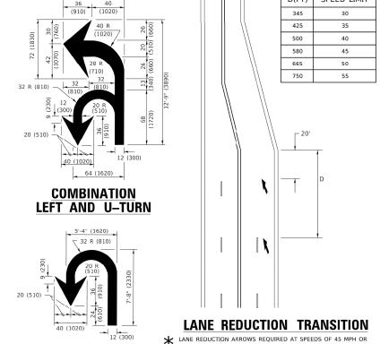
\* LANE REDUCTION ARROWS REQUIRED AT SPEEDS OF 45 MPH OR GREATER OR WHEN SPECIFIED IN PLANS.
