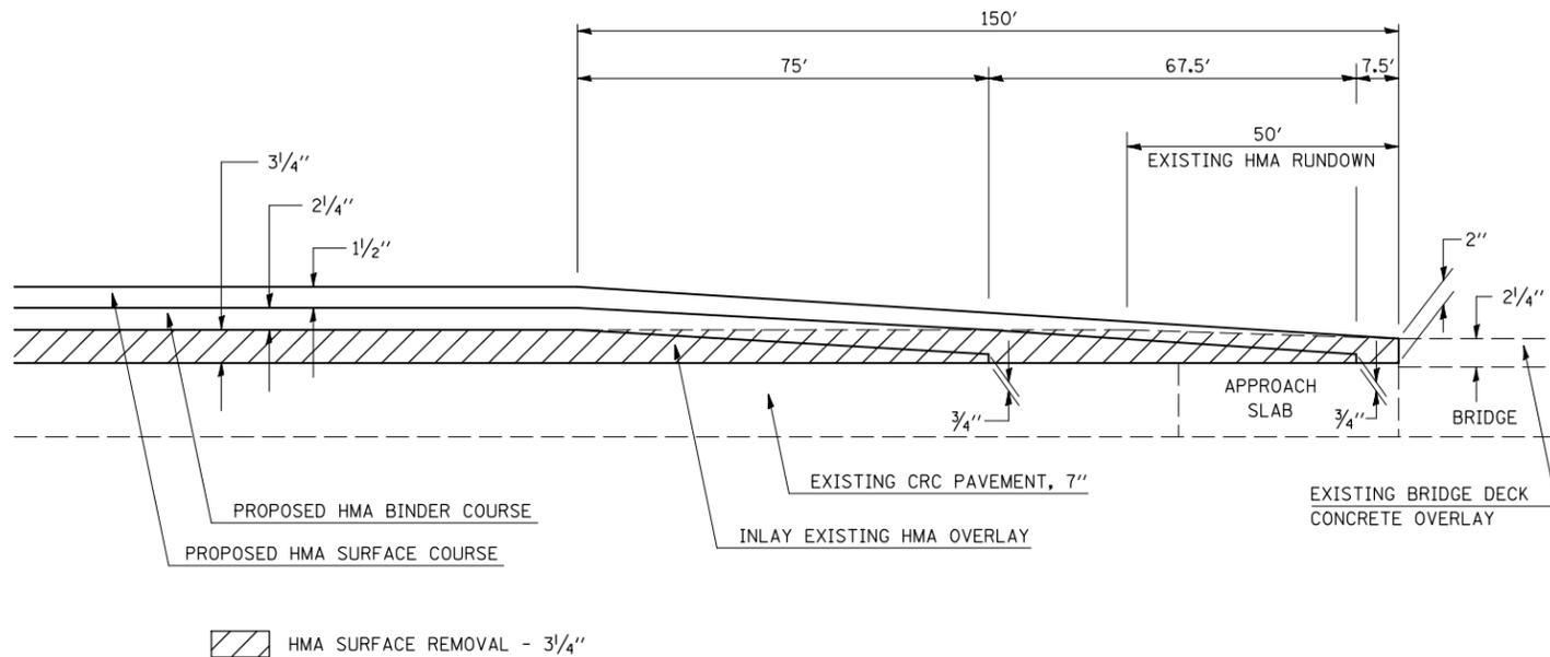
**DETAIL OF BUTT JOINT - DRIVING LANE**
