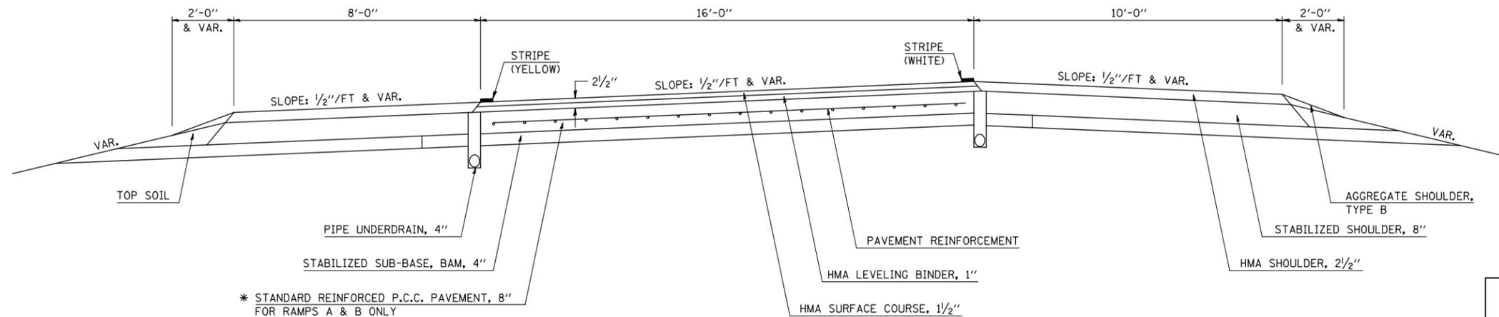
\* NOTE: RAMPS C & D HAVE CONTINUOUSLY REINFORCED P.C.C. PAVEMENT, 8"
