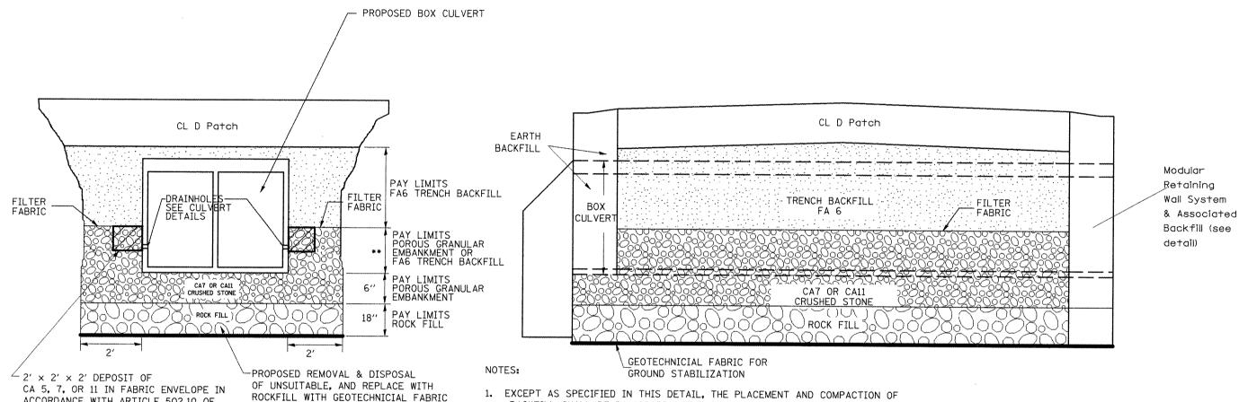
\*\* EXTEND THE POROUS GRANULAR EMBANKMENT TO THE TOP OF THE DRAINHOLE FILTER FABRIC ENVELOPES.
