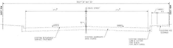
PAVEMENT WIDTH VARIES FROM 17± TO 13± FROM STA 21+06.18 TO STA 21+59.44
