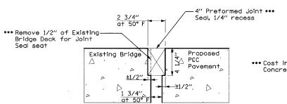
\*\*\* Cost included with Portland Cement Concrete Pavement 7" (Jointed)
