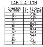
THE CONCRETE COLLAR SHALL BE PAID FOR AT THE CONTRACT UNIT PRICE PER CUBIC YARD FOR **CONCRETE COLLAR,** AS SHOWN ON THE PLANS, WHICH PRICE SHALL INCLUDE THE REMOVAL OF SUCH PORTIONS OF THE EXISTING HEADWALLS AS MAY BE REQUIRED.
