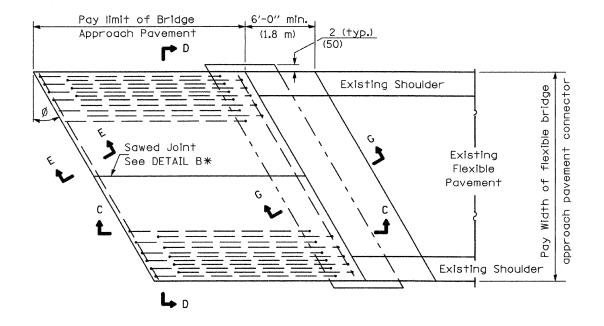
BRIDGE APPROACH PAVEMENT CONNECTOR (FLEXIBLE)
