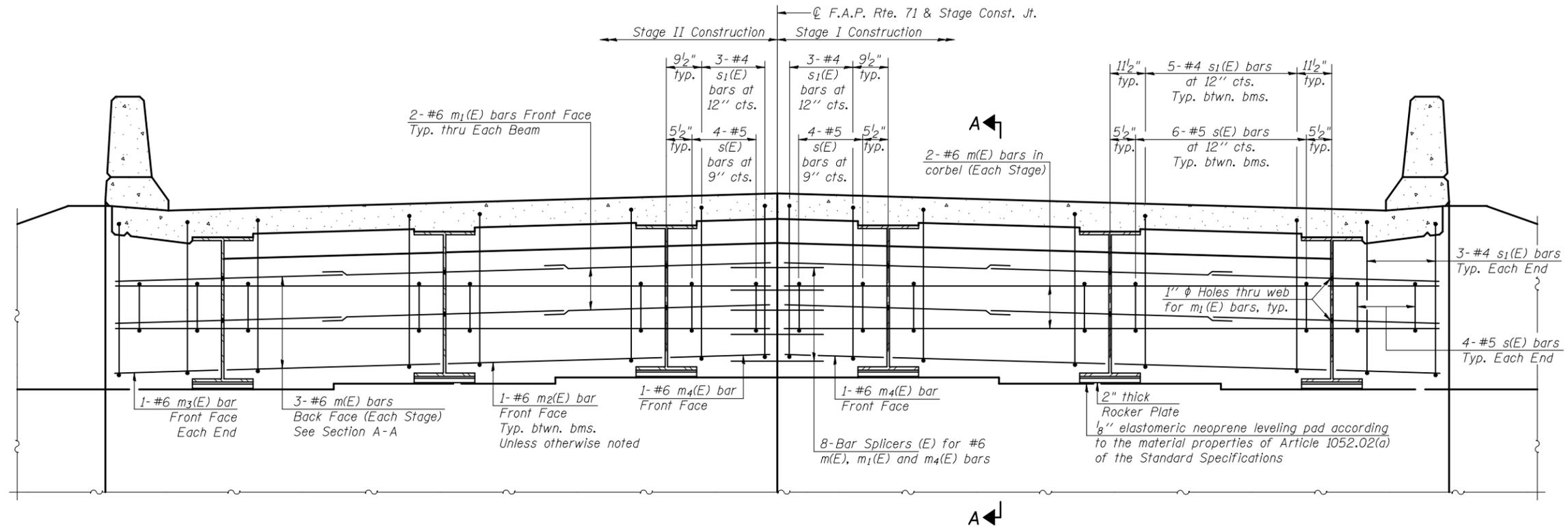
**DIAPHRAGM ELEVATION AT ABUTMENT**
