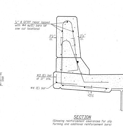
½″ ¢ GFRP rebar, 4'-6" long. -ex (Е) d(E)saw cut
