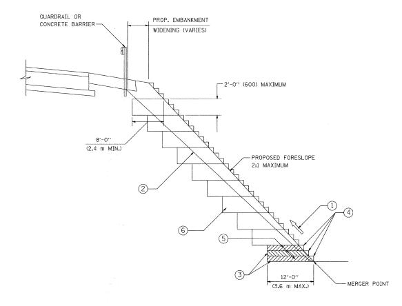
TYPICAL BENCHING DETAIL FOR EMBANKMENT
