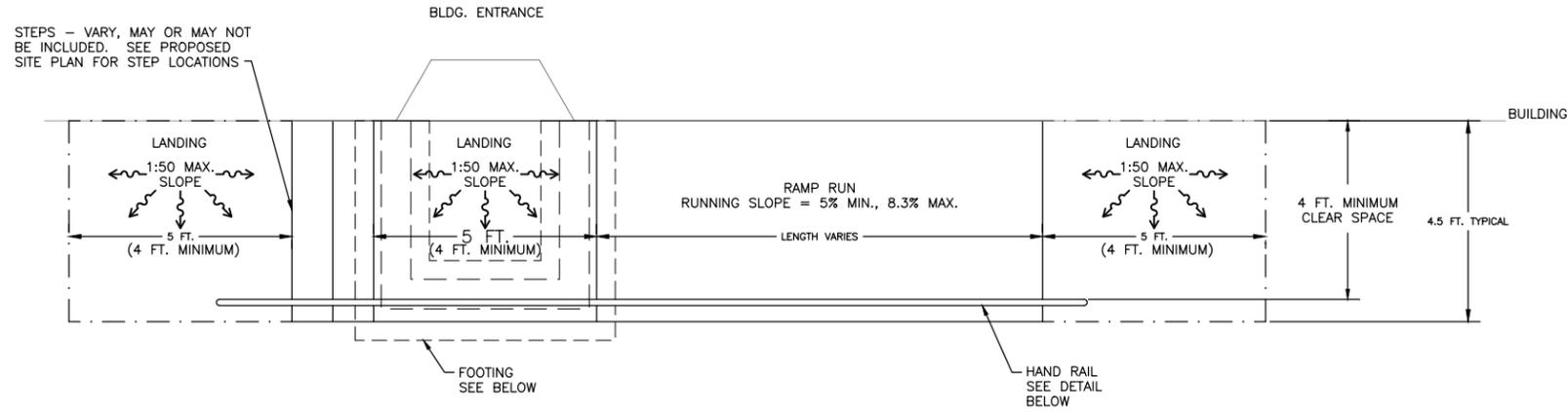
**ADA ACCESS RAMP STANDARD TYPICAL DETAIL**
