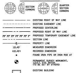
STAKING OF PROPOSED RIGHT OF WAY CORNERS. SET 5/8 INCH METAL ROD WITH DIVISION OF HIGHWAY SURVEY ALUMINUM CAP TO MONUMENT THE POSITION SHOWN. IDENTIFIED BY INSCRIPTION DATA AND SURVEYORS LICENSE NUMBER. (PROPOSED RIGHT OF WAY CORNERS SET IN CULTIVATED AREAS SHALL BE A MINIMUM OF 20 INCHES BELOW THE GROUND SURFACE).
